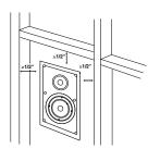
3. **NOTE:** Always allow at least a 1/2 inch between a wall stud and the speaker cutout or the locking tabs will not be able to swivel into place.
